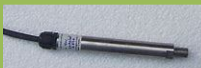
VW Sensor for Uplift Pressure Meter
